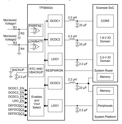
Figure 7. TPS65023 Simplified Application Circuit
