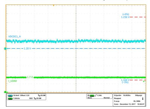
Figure 16. VDCDC1\_A Full Load Test
