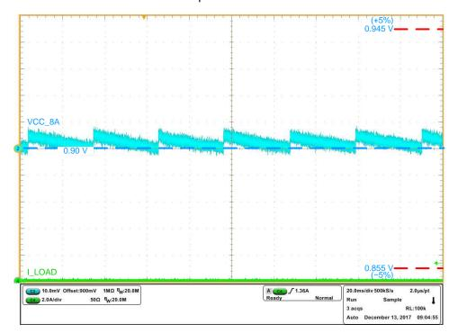
Figure 18. VCC\_8A No Load Test
