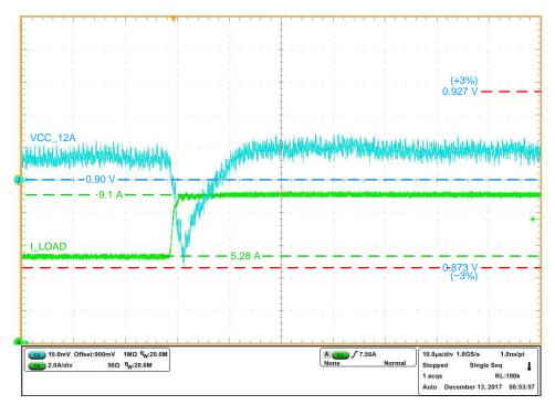
Figure 23. VCC\_12A Load Step Test
