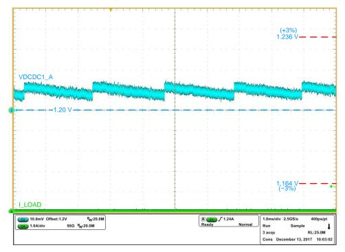
Figure 15. VDCDC1\_A No Load Test
