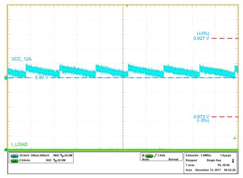
Figure 21. VCC\_12A No Load Test
