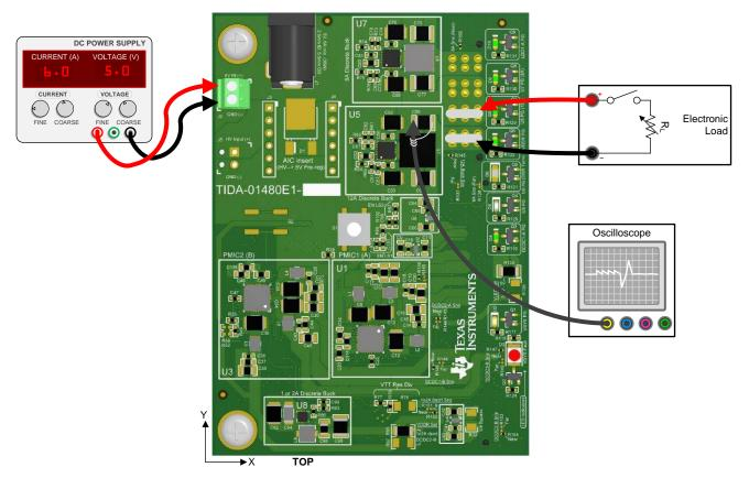
Figure 14. Setup for Measuring Output Voltages with Load Applied
