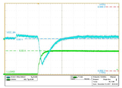
Figure 20. VCC\_8A Load Step Test
