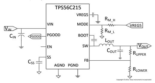
Figure 8. TPS56C215 Simplified Application Circuit
