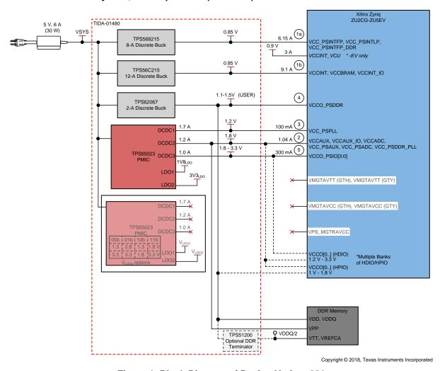
Figure 1. Block Diagram of Design Variant 001
