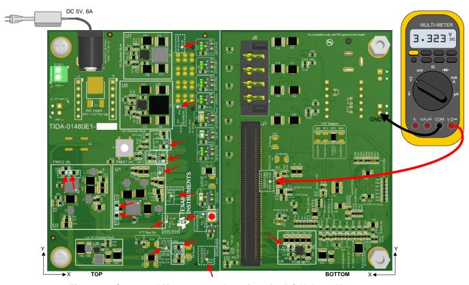
Figure 13. Setup and Measurement Locations for DC Voltage Measurements
