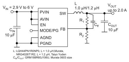
Figure 9. TPS62067 Simplified Application Circuit
