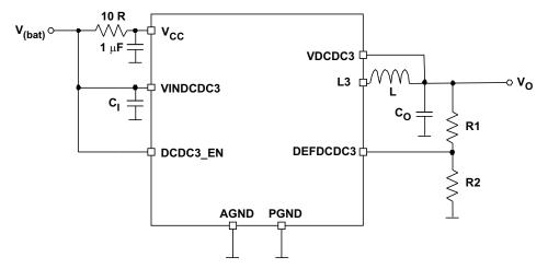
Figure 12. TPS65023 External Resistor Divider for DCDC3
