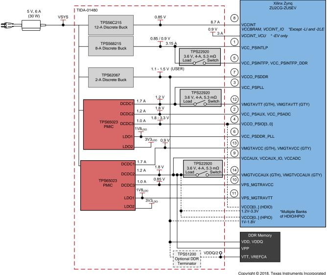
Figure 5. Block Diagram of Design Variant 005
