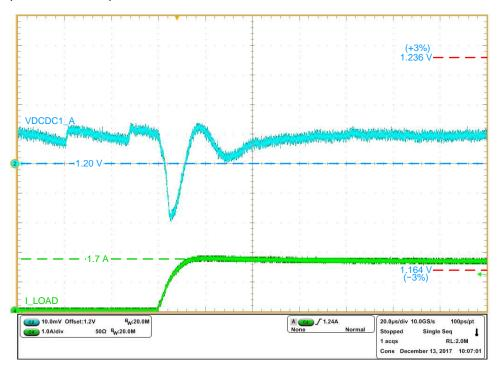
Figure 17. VDCDC1\_A Load Step Test
