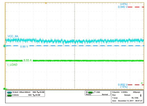
Figure 19. VCC\_8A Full Load Test
